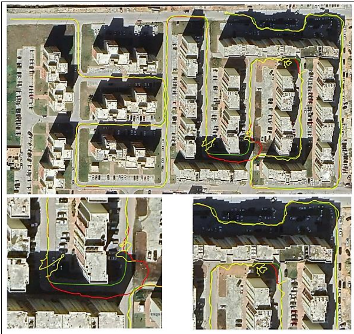
Figure 7 E-PPP and EPPP-NS, in high multipath area
